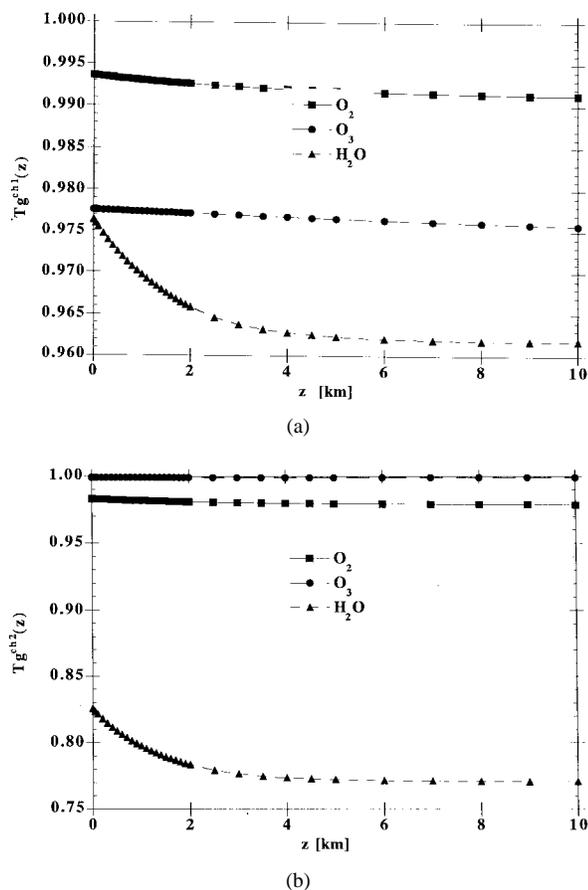
Fig. 11. Variation of the gaseous transmission ( $Tg$ ) as a function of the observer altitude,  $z$ , (airborne case), for AVHRR channel 1(a) and 2(b) spectral responses. The sun zenith angle is  $30^\circ$  and the view zenith angle is  $30^\circ$ . Tropical atmosphere was used.
