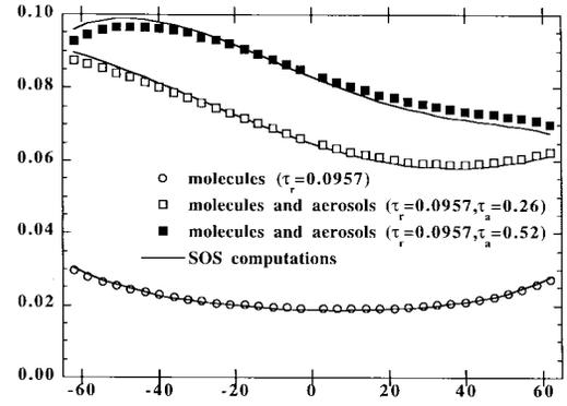
Fig. 6. Comparison of the sum of the coupling terms atmosphere-BRDF:  $\rho_{TOA} - (\rho_{R+A} + e^{-\tau^m} \rho_s)$  computed by 6S with the same quantity computed by the SOS code for different atmospheric conditions (clear, average, turbid). The ground BRDF is from Kimes measurements over a plowed field fitted with Hapke BRDF model.
