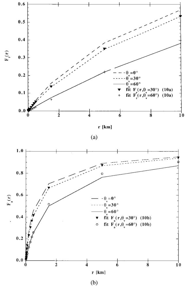
Fig. 4. (a) Environment function for a pure molecular atmosphere (lines) for different view zenith angle ( $\theta_v$ ) compared to approximation used in 6S (symbols) as a function of the distance to the imaged pixel ( $r$ ) and (b) same as (a) but for aerosol.
