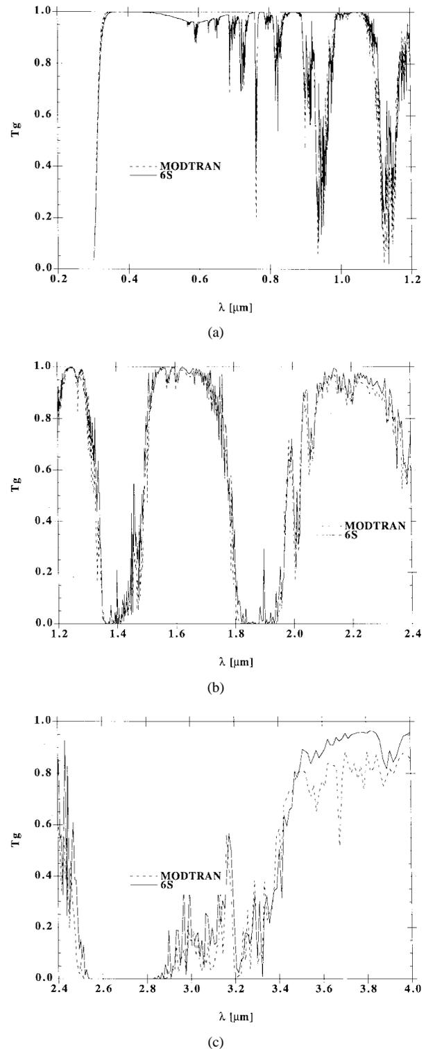
Fig. 13. (a) Comparison of gaseous transmission between 0.20–1.20  $\mu\text{m}$  computed by MODTRAN with the results of 6S for a typical mid-latitude summer atmosphere. (b) Same as (a) but between 1.20–2.40  $\mu\text{m}$ . (c) Same as (a) but between 2.40–4.0  $\mu\text{m}$ .
