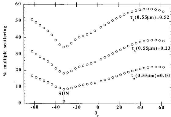
Fig. 1. Contribution of multiple scattering to the intrinsic aerosol reflectance as a function of the view zenith angle for several aerosol optical depth in case of a continental aerosol model for AVHRR channel 1. Computations are performed for two relative azimuths ( $\phi = 0^\circ$  for  $\theta_v < 0$ ,  $\phi = 180^\circ$  for  $\theta_v > 0$ ).
