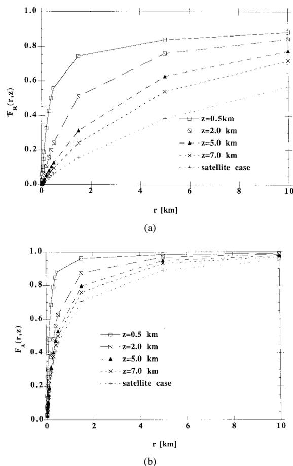
Fig. 12. (a) Variation of the molecular environment function, ( $F_R$ ) for different altitude of the sensor. (b) Variation of the aerosol environment function, ( $F_A$ ) for different altitude of the sensor.
